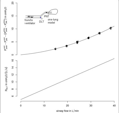
**Fig. 1** Measured and modelled pressure drop over double-lumen tube (DLT) resistance from ventilator ( $P_{\text{ven}}$ ) to tracheal ( $P_{\text{trach}}$ ) measured using a pneumotachograph (PNT) side of the DLT as well as corresponding DLT resistance ( $R_{\text{DLT}}$  lower row) over airway flow
