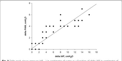
**Fig. 3** Delta peak airway pressure (pP<sub>AW</sub>) in centimeter of water as a function of delta IAP in centimeter of water. Delta pP<sub>AW</sub> =  $0.14 + 0.43 \times \text{delta}$  IAP,  $R^2 = 0.83$ , p < 0.001
