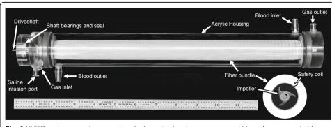
**Fig. 1** ULFED prototype and cross-sectional schematic showing arrangement of impellers surrounded by safety coil and annular fiber bundle
