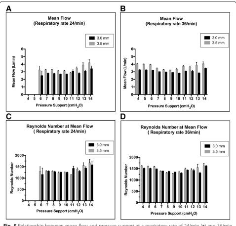
**Fig. 5** Relationship between mean flow and pressure support at a respiratory rate of 24/min (a) and 36/min (b). Relationship of Reynolds number and pressure support at a respiratory rate of 24/min (c) and 36/min (d) (p < 0.05 by Tukey's multiple-comparisons test). Error bars represent standard deviation values
