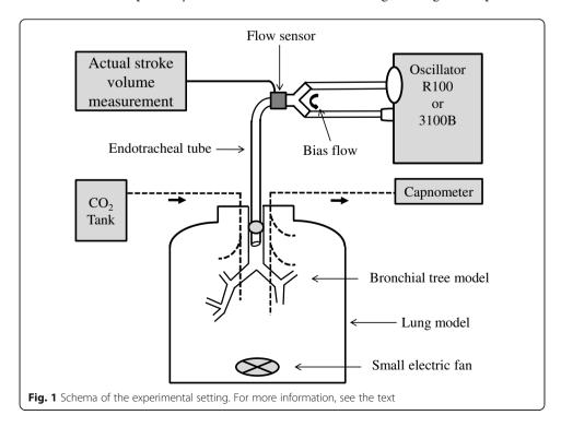
were as follows: MAP of  $25 \text{ cmH}_2\text{O}$ , BF of 30 L/min, and fraction of inspired oxygen of 0.21. The heated humidifier was turned off (hollow fiber type, R100) or removed from the circuit (chamber type, 3100B).
