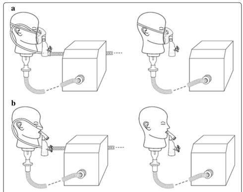
**Fig. 2 a** A facemask, utilized with an aerosol chamber positioned on an adult head model, was connected to a breathing simulator via a collecting filter, with and without concurrent HFNT. **b** A mouthpiece, utilized with an aerosol chamber positioned on an adult head model, was connected to a breathing simulator via a collecting filter, with and without concurrent HFNT. The VMN was positioned in the aerosol chamber
