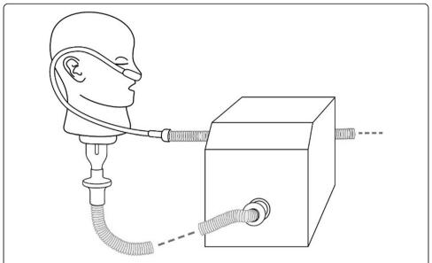
**Fig. 1** High-flow nasal cannula was positioned on an adult head model, which was connected to a breathing simulator via a collecting filter. The VMN was positioned at the humidification chamber
