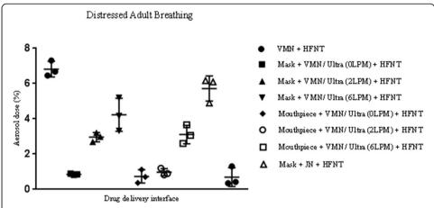
**Fig. 5** Illustration of aerosol dose (percentage) for each delivery modality with concurrent HFNT, during simulated distressed adult breathing. The values represented are mean  $\pm$  standard deviation (expressed in percentage) of three independent experiments
