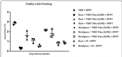
**Fig. 4** Illustration of aerosol dose (percentage) for each delivery modality with concurrent HFNT, during simulated healthy adult breathing. The values represented are mean  $\pm$  standard deviation (expressed in percentage) of three independent experiments
