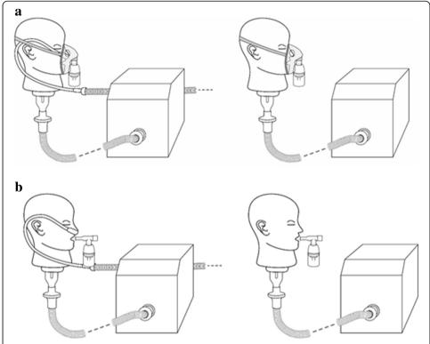
**Fig. 3 a** A facemask, positioned on an adult head model, was used with a jet nebulizer and was connected to a breathing simulator via a collecting filter, with and without concurrent HFNT. **b** A mouthpiece was used with a JN and was connected to a breathing simulator via a collecting filter, with and without concurrent HFNT
