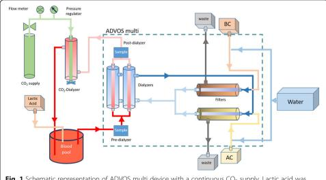
Fig. 1 Schematic representation of ADVOS multi device with a continuous  $CO_2$  supply. Lactic acid was supplied in blood only for experimental settings 2 and 4 (see Table 1 for more details)
