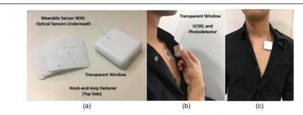
**Fig. 2 a** Wearable sensor and patch,  $\bf b$  side view use of the wearable platform, and  $\bf c$  front-view use of the wearable platform
