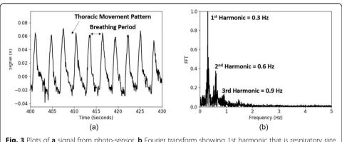
**Fig. 3** Plots of **a** signal from photo-sensor. **b** Fourier transform showing 1st harmonic that is respiratory rate and the multiple higher-order harmonics
