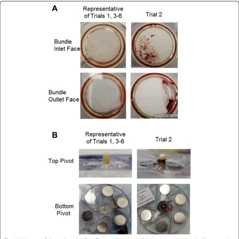
**Fig. 4** (a) Images of the explanted hollow fiber membrane bundle inlet (*top row*) and outlet (*bottom row*) faces and the (b) impeller top (*top row*) and bottom (*bottom row*) pivots. The animal 2 (*right*) bundle and pivots had significant thrombus formation due to low ACT. All other animals were free of significant thrombi (*left*)
