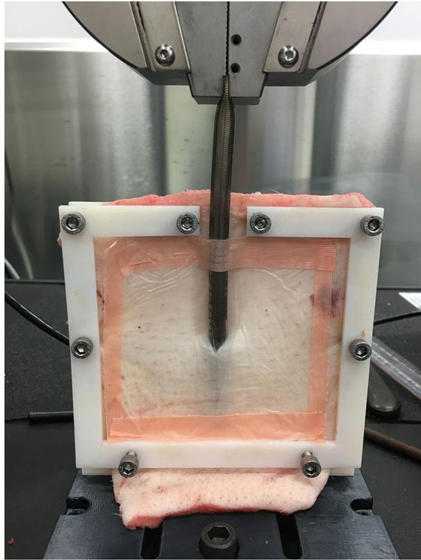
**Fig. 1** Secured cannula on the Instron 5567 Universal Testing System
